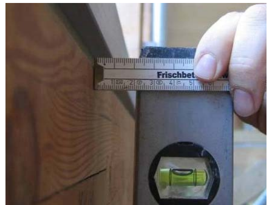
Fig. 6: Rotation of Lower Flange
