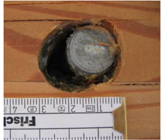
Fig. 4: Indentation of Dowel into Timber
